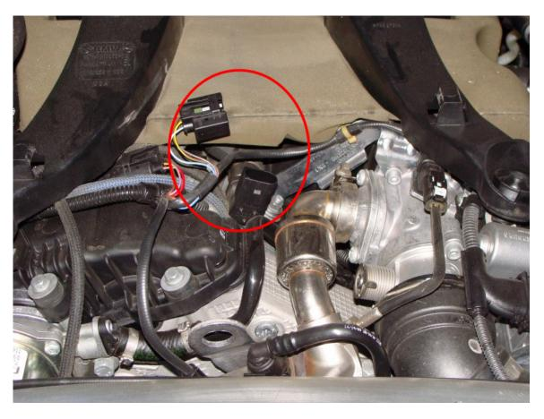
Insert the JBD male connector in to the OEM female connector as shown. Take care to ensure it is fully inserted and the retaining clip closed over the tab.
