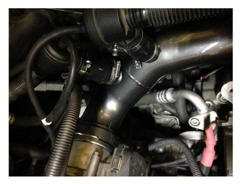
9. Reinstall the factory intake by reconnecting and fastening the 2 inlet tubes and pushing down on the box to seat the 3 rubber retainers.
