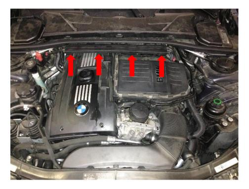
2. Remove the lower part of the cable cover from the cowl. You may need a small screwdriver to push the clips down to release the 3 latches. Once the cover is loose, unclip the wires and remove the cover.
