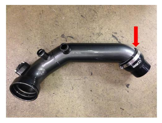
4. Install the COBB Charge Pipe on the car first seating the throttle body section. Once seated, install the stock C-Clip to secure the pipe in place. Install the C-Clip in the same orientation used on the stock charge pipe.
