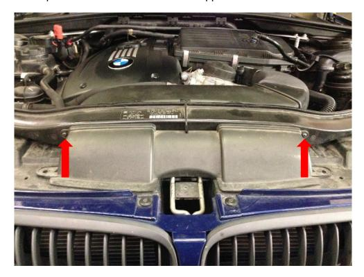
13. Reinstall the lower part of the cable cover to the cowl and re-secure the cables into the cover.
