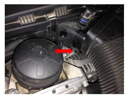
8. Pull up on the airbox to remove it. There are 3 rubber retainers holding the airbox to the engine.
