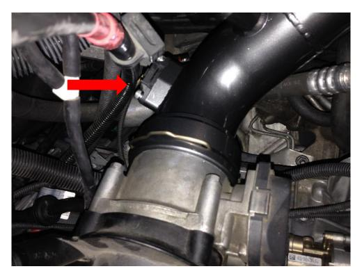
6. Slide the silicone reducer over the aftermarket or stock intercooler pipe and tighten the 040 hose clamp with an 8mm socket or nut driver.
