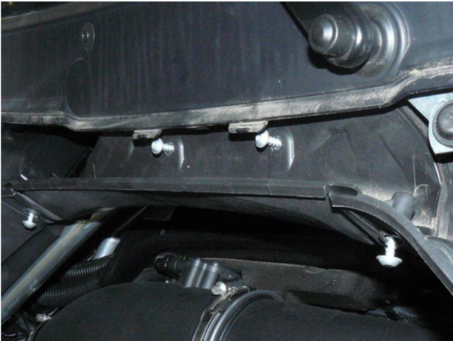
Remove the 4 screws and carefully lift out the center partition wall.
