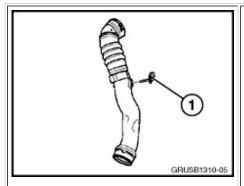
Replace the charge air temperature sensor (1) (refer to Repair Instruction RA 13 62 538).
