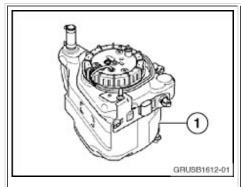
Replace the SCR active tank (1) (refer to Repair Instruction RA 16 19 020). Fill the new tank with new diesel exhaust fluid (DEF)
