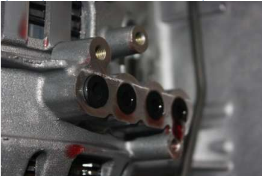
Figure 16 The 4 Sealing Sleeves Replace while its easy
