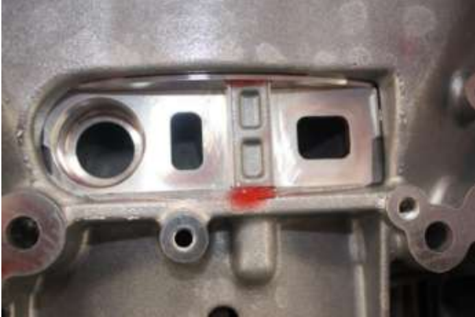
Figure 15 Bridge Seal adapter Fits Here. This seal is Prone to Cracking
