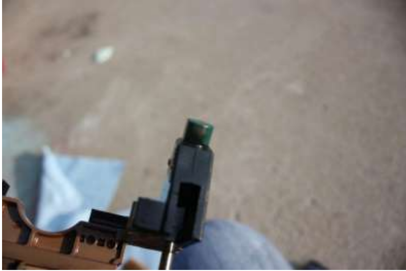
Figure 13 Take a look at this ISS Sensor. It is covered in Fine Metal which affects the readings! Clean it off
