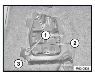
Release nuts (1), tightening torque 63 21 1AZ.
