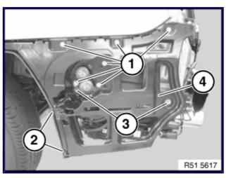
If necessary, unlock and disconnect plug connection on RDC trigger transmitter.
