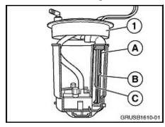
If the DEF level in the active tank (1) is above the full point (A) of the level sensor, the fluid level reading will be at 100% (full). Once the DEF level is below the full point of the level sensor, but still above the warning point (B), the level reading will be 66%. The warning scenario displayed to the customer will start to count down the mileage to "no start condition" when the DEF level is below the warning point (B), and above the empty point (C) of the sensor.
