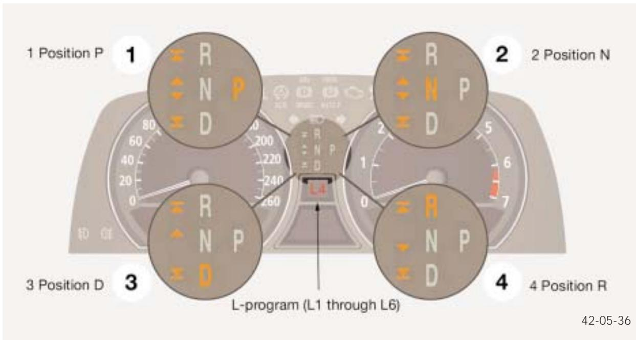
After switching on the ignition and starting the engine, the P or N positions and all of the arrows are indicated. In positions D or R, the single arrow for the shift direction to return to N is indicated (next to the N indicator).
