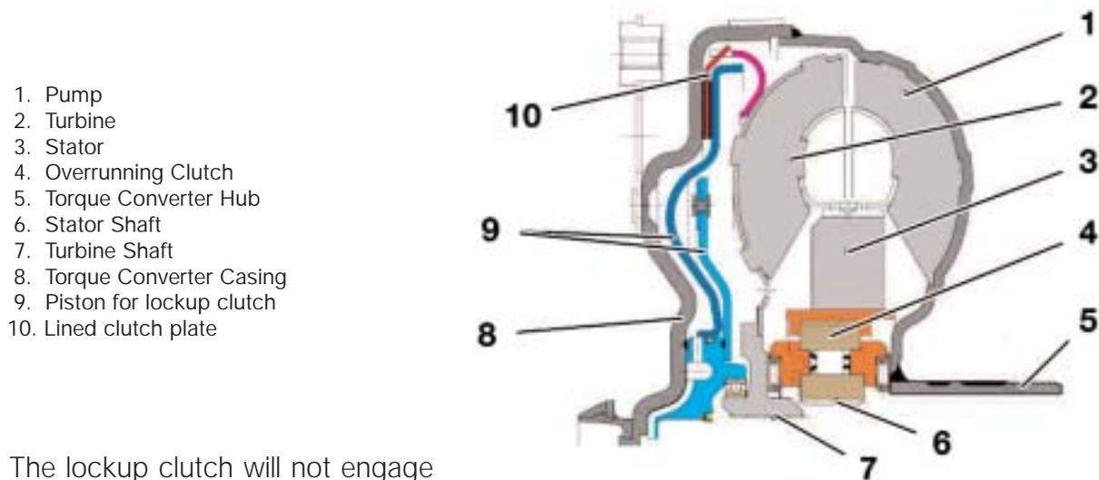
The lockup clutch will not engage until the oil temperature is  $>35\text{ }^{\circ}\text{C}$ . The control of the lockup clutch depends on various factors such as:
