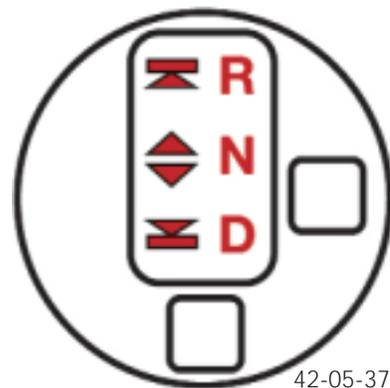
The **position indicator** for R, N or D is highlighted corresponding to the engaged gear position (position D is highlighted here). The positions are indicated when the ignition is "ON" and the transmission is not in position P.
