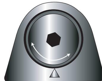
***Do not overtighten the drain plug because the plug and oil pan will distort or crack!***
