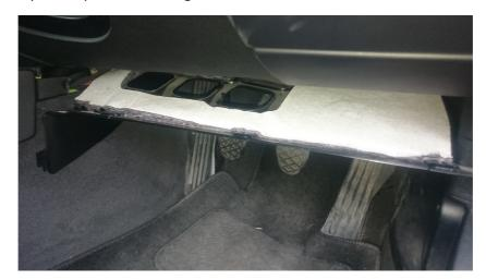
Going from the footwell trim you should now be able to run the cable up to the top of the airbag pillar and put the mic right in the top corner of the windscreen. Once you're happy with the location peel off the cover for the M3 tape and stick it to the windscreen. Once stuck you can now run the cable behind the velvet cover highlighted by the red line in the image below. Once happy screw the airbag pillar back in place.
