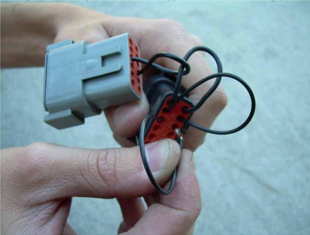
When done, it should look like this - three loops, **(1-12)** **(2-11)** **(3-10)** and if you are running the **Speed Limit Defeat** a fourth loop needs to be installed - **(4 - 9)**
