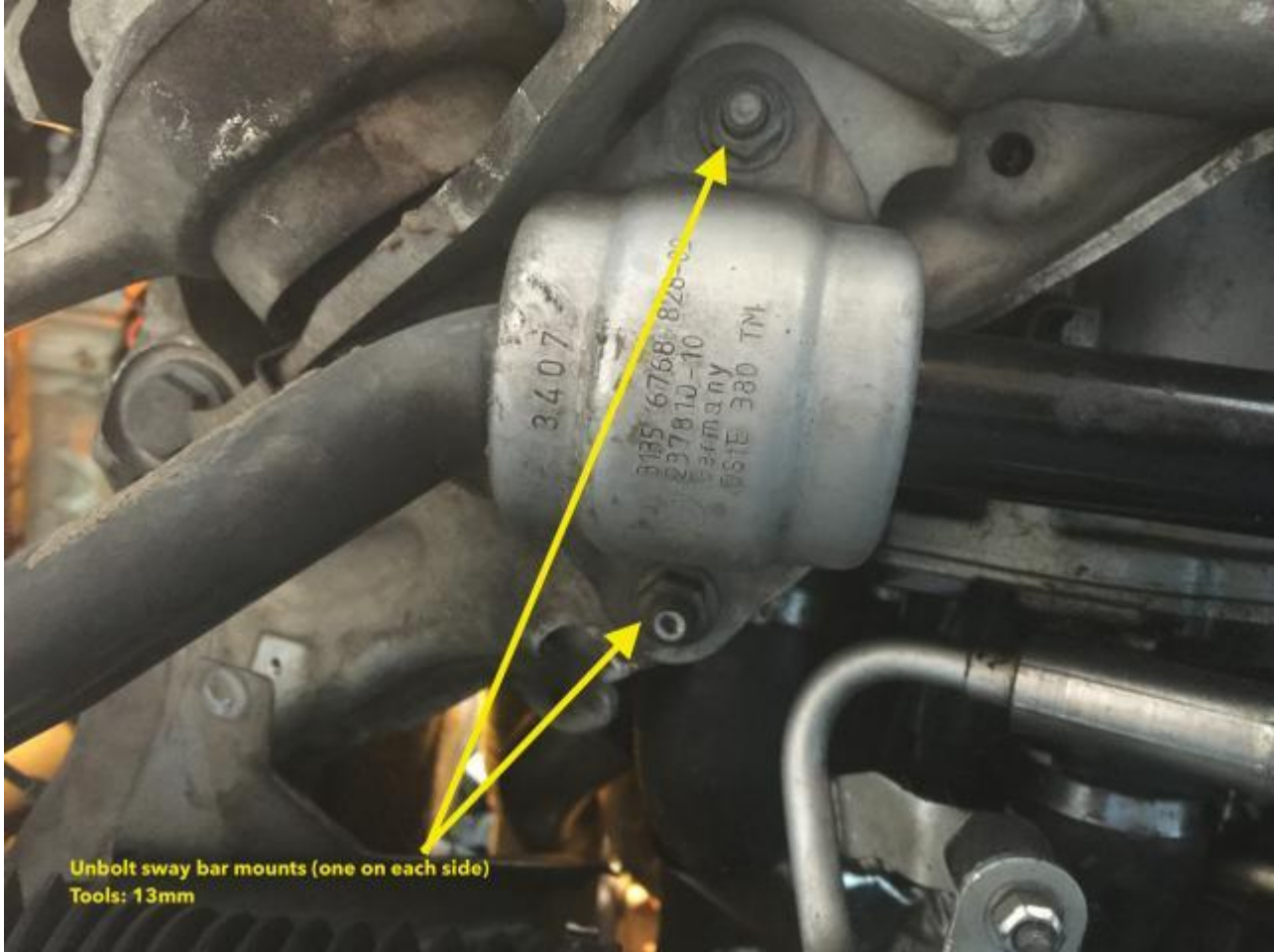
Unbolt sway bar (one on each side) Tools: 17mm x2
