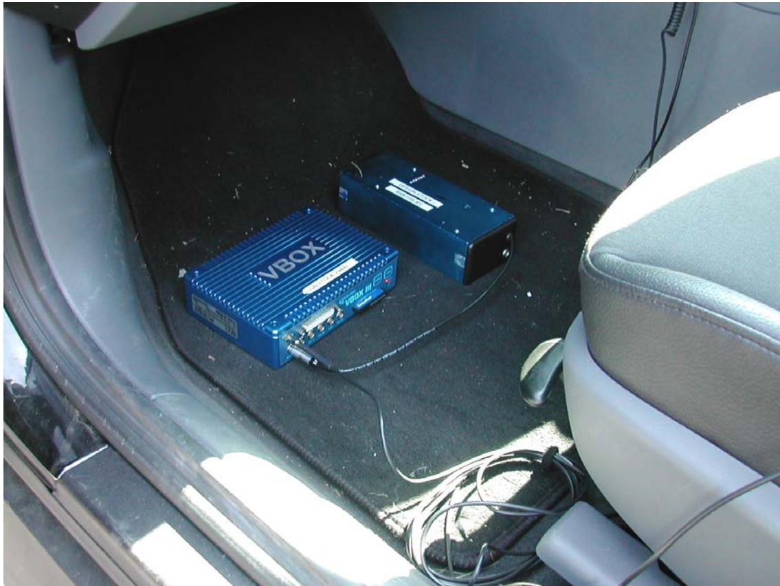
Placement of VBox III in passenger footwell
