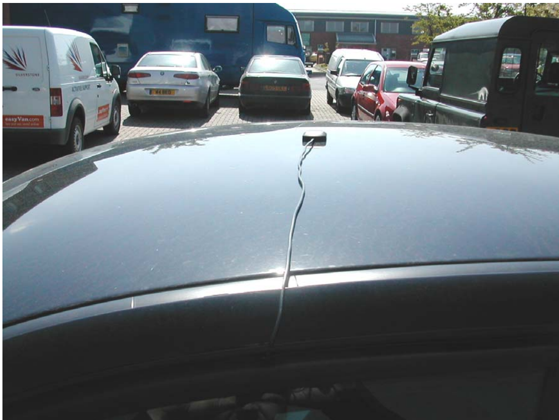
Placement of VBox III external GPS antenna
