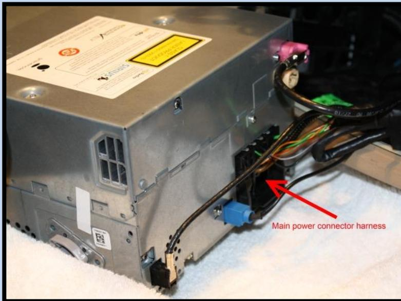
1. Please locate the main power connector harness at the back of the head unit, as shown on the picture on the left.
