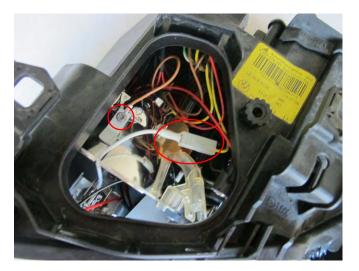
57. Replace top Cover on headlight and take both completed headlights to the car for testing do not attempt to install the lens on the headlights yet. Carefully secure headlights and plug in wire harness. Test all headlight functions (note turn signal bulb has been removed).
