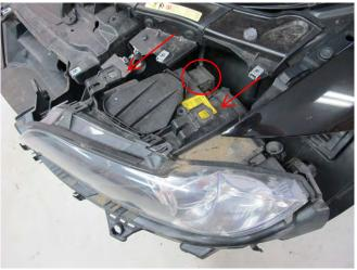
15. Remove the two T-30 Torx from each headlight bracket that secures the headlight to the mounting bracket then remove bracket.
