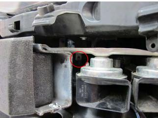
11. (Non M3 Only) Locate the lower brace attaching the bottom of the headlight back to the chassis of the car. The rear portion of the plastic brace is slip connected to the car. Typically you can pull down firmly on this end and it will disconnect. If you have a side that is being stubborn take a long flat blade screw driver and pry open the mouth of the brace where it slips over the chassis while pulling down to release it.
