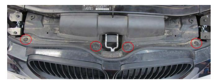
9. Carefully remove front bumper cover and place out of the way sitting up so it does not get damaged.
