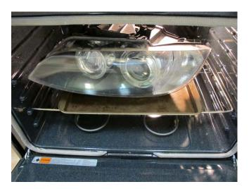
20. Remove headlight with gloves so that you can handle the headlight without getting burned.
