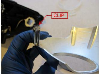
31. Holding the cornering light housing assembly carefully the upper clip on the clear lens to release it then release the lower clip removing the corner light reflector housing and clear halo ring.
