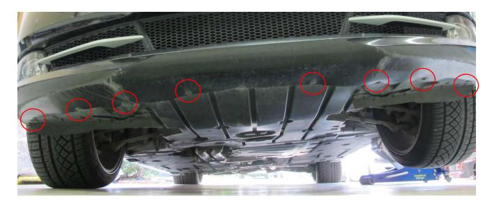
4. Turn the steering wheel to gain access and remove the 8mm bolts inside the finder liner which secure the liner to the bumper cover (for m3 remove the two 10mm plastic nuts on driver's side and two 8mm plastic nuts on passenger side).
