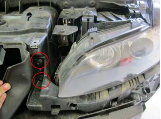
14. The top two T-30 Torx on each headlight is all that is left holding them to the car. Carefully remove the screws while holding the headlight. Once they are out remove the headlight and disconnect the wiring then carefully place the headlights on a towel or other soft material to keep lens from getting scratched.
