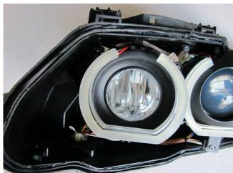
64. Put a little water on a paper towel and dab your finger on it as needed while you push the sealant into the headlight channel. Work your way around the entire channel making the sealant as wide as possible and with little to no voids.
