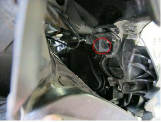
13. Remove the two T-30 Torx from the inside of each headlight closest to the air supply for radiator.
