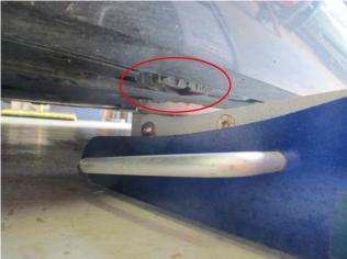
3. Remove the 8mm bolts holding the lower bumper cover to the plastic under tray of the car.
