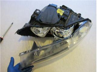
24. Using your hand grab onto the wires next to the plug inside the lens wiggle and pull to remove the plug from the board. The lens will now be free of the assembly and should be placed outside of lens down on a soft towel.
