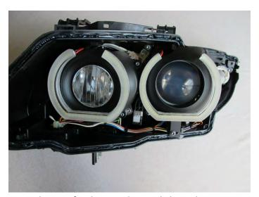
54. Route the wire for the outside DTM light to the top access cover and pull the harness up from the cornering light where it came in through the factory bulb location.
