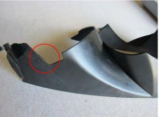
61. Install the Carbon Fiber eyelid inside the lens it is not secured by glue or tape of any kind it fits loose until everything is assembled. For now insert between the turn signal lens and the headlight lens on the inside.
