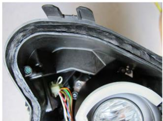
65. Carefully install headlight lens it is a very tight fit with the new rings do not force it. As you line things up and push the lens on watch for clearance between the projector ring and the housing for the cornering light. We left an 1/8" gap earlier for this reason we need some clearance. Also watch around the cornering light DTM ring and make sure it doesn't snag. Everything will fit just take a little time and don't force it things needs to line up as you push them together.
