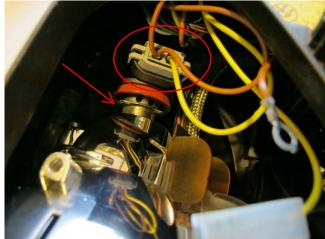
28. Remove the single T-15 Torx screw from the metal brace inside the access cover (Will have brown ground wire attached as well with this screw).
