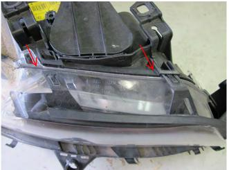
17. Pull the rubber vent in the corner of each of the headlights and remove them. Twist and remove the turn signal bulb from the housing. Remove the T-15 Torx that was hidden behind the rubber vent before it was removed.
