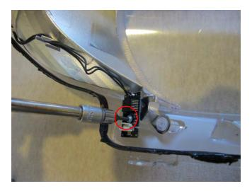
60. Using a dremel or other grinding tool remove plastic from the black shroud that goes inside the lens as shown in the images below. This is required to provide proper clearance for the DTM halo mount.
