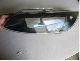
63. The OEM sealant provided in the kit is too thick for the lens to go back on the headlight. Stretch the sealant (making it thinner) as you insert into channel. When stretched correctly there will be a little extra left over. The goal here is to push it into the channel that was created in the old sealant when the lens was removed.
