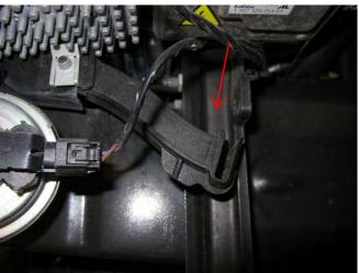
12. Locate and remove the T-30 Torx at the back corner of the headlight just inside the fender (pull back fender liner as needed).
