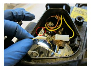
29. Remove the four T-15 Torx screws around the cornering light housing, once removed the front half of the corner light housing can be pulled free (do not remove the rear half of the housing it is not needed).
