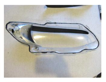
62. Reinstall the black trim inside the headlight housing, tighten all 3 screws tight the back each off ¼ of a turn this will allow for some movement during assembly if the grinding was not done exactly right on the black trim. It will not ever loosen more or appear loose later.
