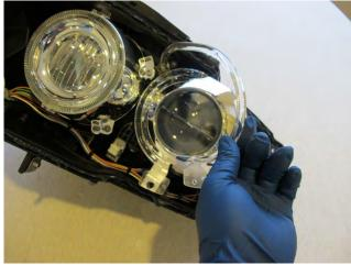
27. Open the top cover and disconnect the cornering light bulb & the plug for the factory angel eye bulb.
