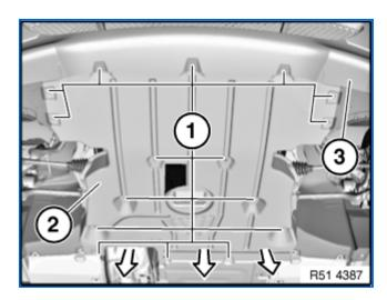
Centre underbody protection (2) and tighten down screws (1).
