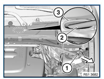
Hold down grommet (3) and pull out left tension strut (2) and right in direction of arrow.
