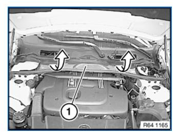
Feed out microfilter housing lower section (1) in direction of arrow and remove.
