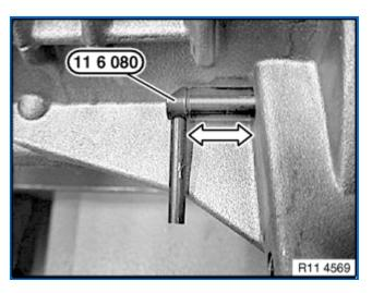
Crank engine at central bolt in direction of rotation until piston of 1st cylinder is in TDC setting.
