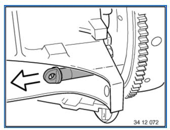
Remove protective cap in direction of arrow.
