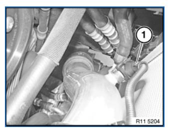
Disconnect plug connection (1) on right pressure pipe.
