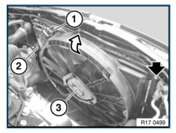
Unlock and disconnect the connector (1).
