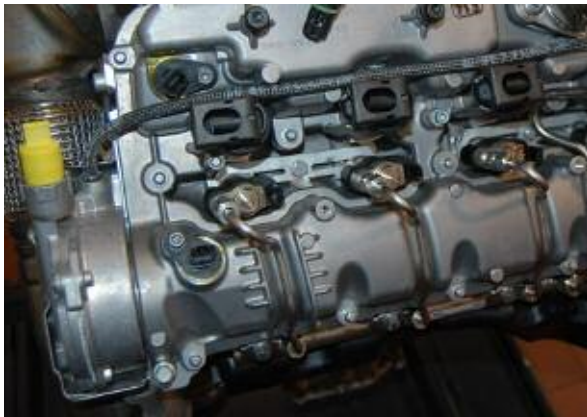
N63 Vacuum pump location
