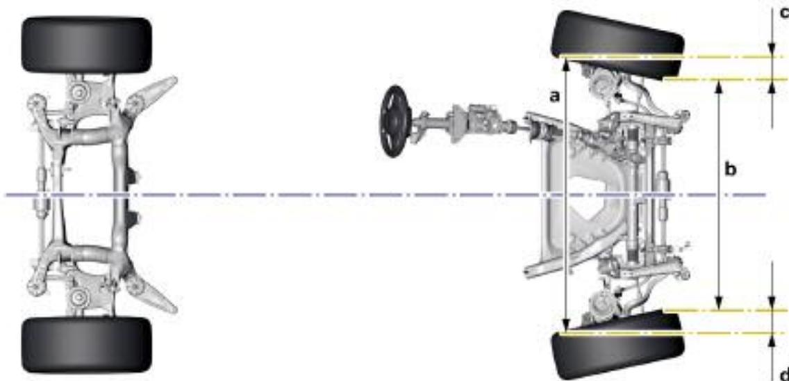
Toe has a major influence on vehicle handling, straight line stability and the position of the steering wheel. An incorrect toe setting will have a negative effect on tire wear. A toe angle which is out of specification will cause the tires to wear in a relatively short time.
