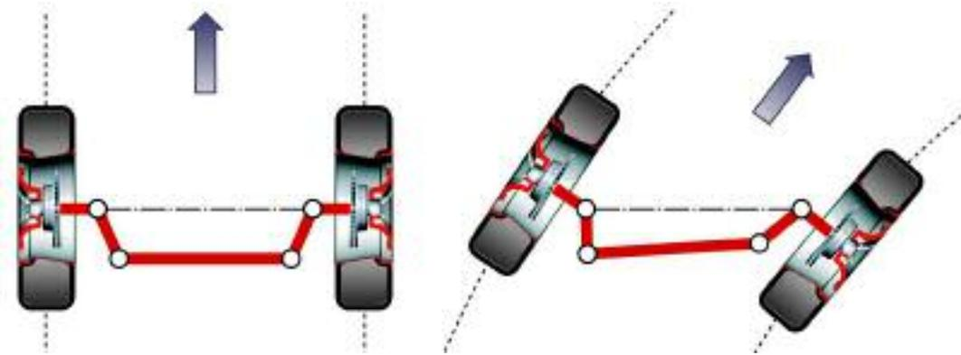
The steering trapezoid enables the steered wheels to be turned at different angles.
