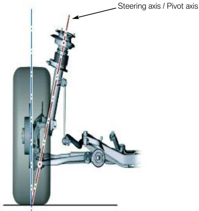
Wheel suspension kinematics can cause this axis to move when the steering angle changes.
