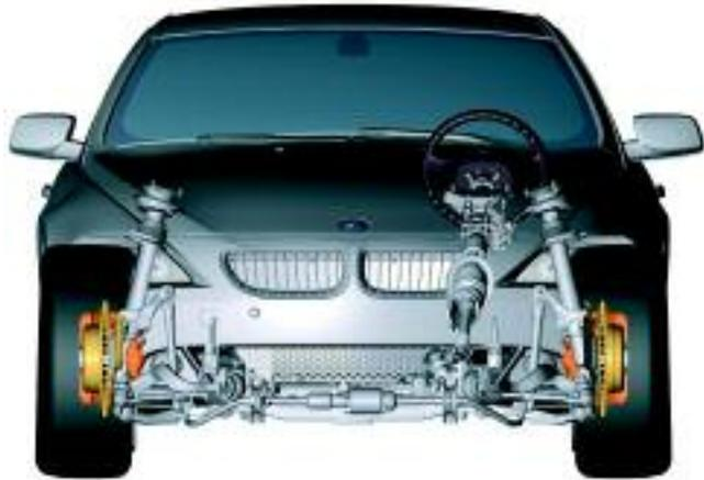
Today, a passenger car steering system is expected to carry out a host of different tasks. It is no longer sufficient just to move the vehicle in the desired direction. The steering process must take function, comfort and safety aspects into account. The vehicle should follow even slight steering movements precisely and on target, without the driver having to make any further corrections at the steering wheel.
