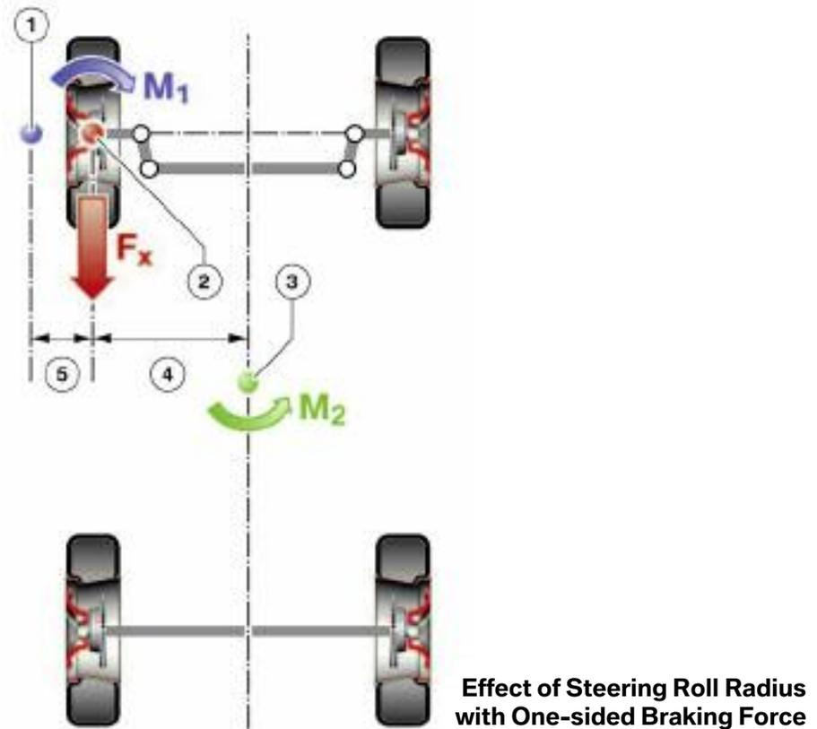
Let us assume that a one-sided braking **force  $F_x$**  is exerted on the left-hand front wheel. It is exerted at a **distance (5)** from the wheel's center of rotation. This distance corresponds exactly to the steering roll radius. A clockwise torque is thereby created on this wheel. If the driver permits it, the steering will therefore be turned slightly to the right.
