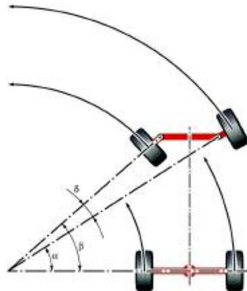
The steering trapezoid enables all wheels to turn about a common cornering center point.
