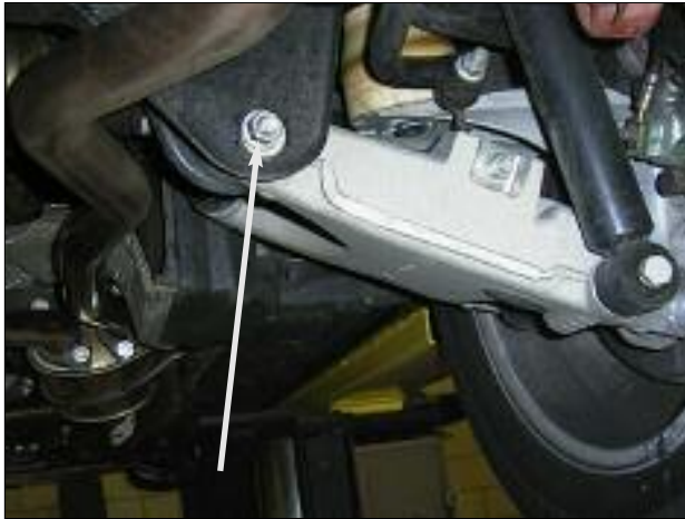
E53 Camber Adjustment (other integral axles similar)
