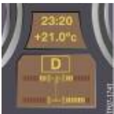
Dynamic Performance Control display with standard longitudinal distribution (front/rear) and lateral distribution biased to the right
