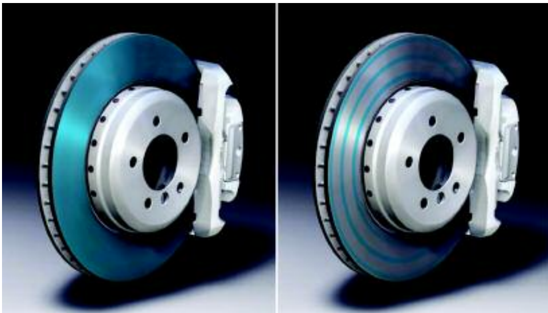
Left disc with water film before dry braking
