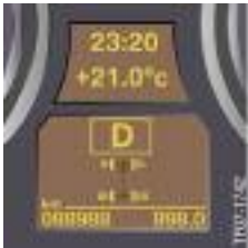
Dynamic Performance Control display with small symbol and odometer reading (displayed upon engine startup)
