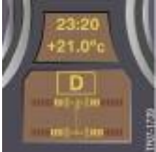
Dynamic Performance Control display with standard longitudinal distribution (front/rear) and even lateral distribution (left/right)
