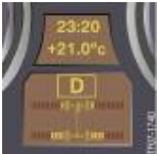
Dynamic Performance Control display with longitudinal distribution biased to the rear and even lateral distribution (left/right)
