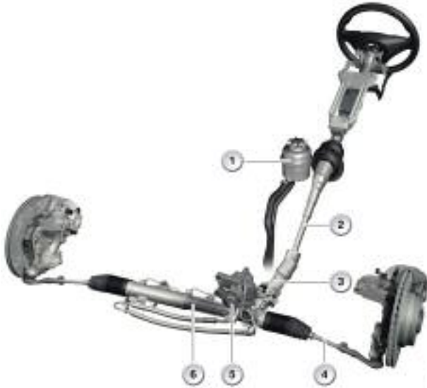
Hydraulic Power Steering (typical installation configuration)
