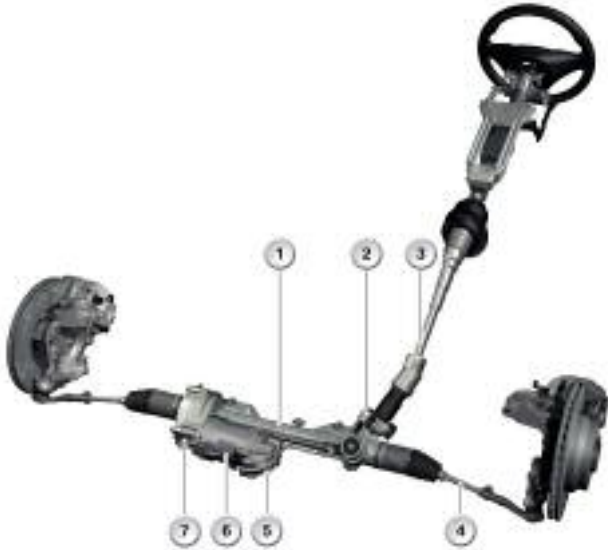
Electric Power Steering with Parallel-mounted Motor
