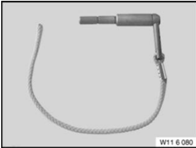
Alignment pin 11 6 080 (used for securing cylinder 1 TDC).
