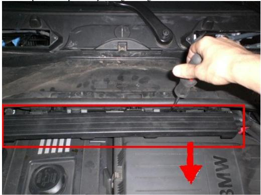
Release the cable bundle using a flat-head screwdriver.
