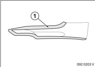
Roughen marked area (1) on inside of front apron attachments with abrasive paper from the Betalink package. Thoroughly clean area with supplied Betalink cleaner.
