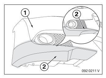
Make sure that the Betalink cleaner does not come in contact with the fog lights, grille and trim. Clean front apron (1) in illustrated area (2) with Betalink cleaner.
