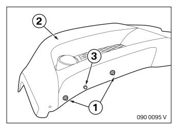
Undo screws (1) on front apron (2). Remove expanding rivet (3).
