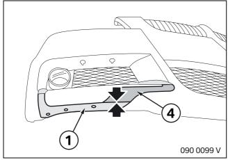
Place adhesive strip **4** exactly against the edge of adhesive strip **1** and adhere in position.
