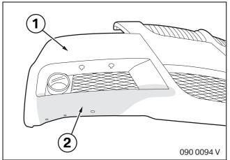
Make sure that the Betalink cleaner does not come in contact with the fog lights, grille and trim. Clean front apron (1) in illustrated area (2) with Betalink cleaner.
