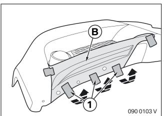
Wrap adhesive tape (1) around lower area of front apron attachment **B**.
