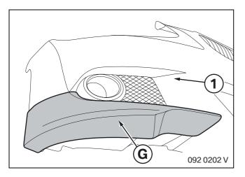
Slightly spread apart the front apron attachment **G** and carefully slide onto the front apron (1).
