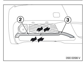
Place adhesive strip **3** exactly against the edge of adhesive strip **2** and adhere in position.
