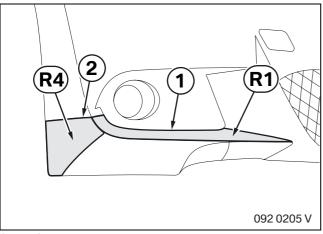
Align adhesive strip  $\ensuremath{\textbf{R1}}$  with marking (1) and adhere in position.
