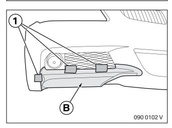
Check the fit of the front apron attachment **B** at all edges and correct if necessary.
