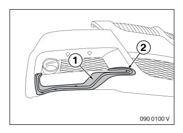
Clean the adhesive strips (1) with Betalink cleaner. Apply a 4 mm diameter bead of Betalink adhesive (2) onto the adhesive strips (1).
