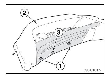
Install screws (1) on front apron (2). Fit expanding rivet (3).
