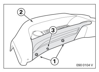
Undo screws (1) on front apron (2). Release underride guard.
