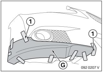
Check the fit of the front apron attachment **G** at all edges and correct if necessary.
