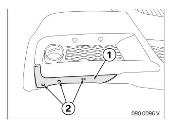
Align adhesive strip **1** with holes (2) and adhere in position.
