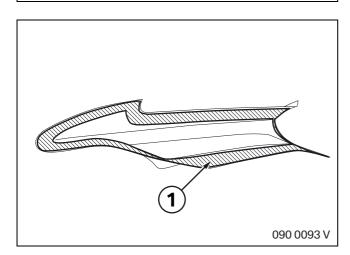
Roughen hatched area (1) on inside of front apron attachments with abrasive paper from the Betalink package. Thoroughly clean area with supplied Betalink cleaner.
