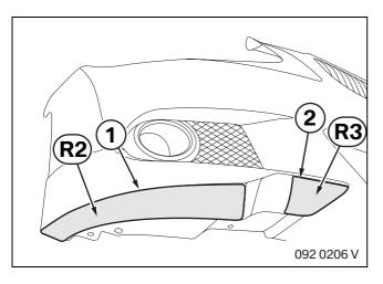
Place adhesive strip **R2** exactly against the edge of adhesive strip (1) and adhere in position.
