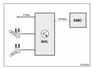
The AHL control unit controls the automatic headlight-range adjustment as follows:
