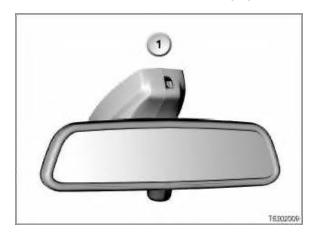
1) Rain-light sensor in base of interior rear-view mirror
