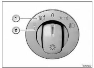
Light switch for vehicles with halogen headlights and manual headlightrange adjustment
