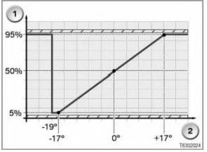
The (Hella) position sensor output signal is a pulse-modulated signal.
