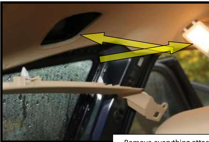
Remove everything attached to the headliner
