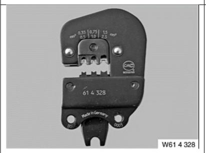
Prior to installing the repair harness into the vehicle, strip the end of the White/Brown wire ,push over the heat shrink tube and crimp one end of the supplied butt connector to the repair harness using crimping tool 614 328 (83 30 0 496 833) Refer to B04 32 06.
