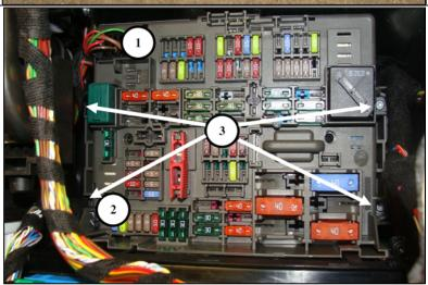
Remove the JBE (Junction Box Electronics) module per repair instructions "61 35 107 Removing and installing or replacing Junction Box electronics".
