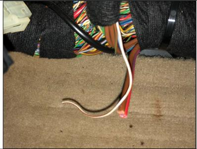
Cut the wiring on the vehicle side for the Red/Violet and Brown wire as close to the main harness as possible (These 2 wires will no longer be used).
