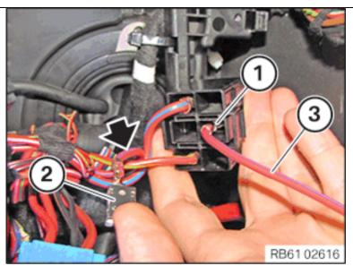
Insert the new wire (1) (3) **Red/Blue**) from the repair harness into the location where the original wire was removed.
