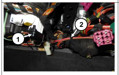
Connect the new repair wire harness connector to the blower regulator (1) Secure the repair cable in place (2) using cable ties along the existing vehicle harness.
