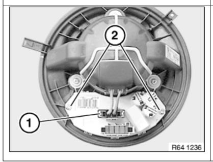
Locate the blower regulator and disconnect **ONLY** the motor connector (1).
