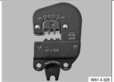
Strip the other end of the vehicle harness White/Brown wire, and crimp to the new wire from the repair harness using crimping tool 614 328 (83 30 0 496 833) Refer to B04 32 06.
