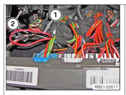
Note: be careful of the sharp edge clip (2) when routing the new harness (1) along the existing vehicle harness.
