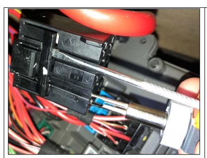
Remove the **Red/Violet** wire from the connector using special tool 61 0 317 from kit (610 300 - P/N 83 30 0 495 382) and a small screwdriver. Refer to SI B04 03 06.
