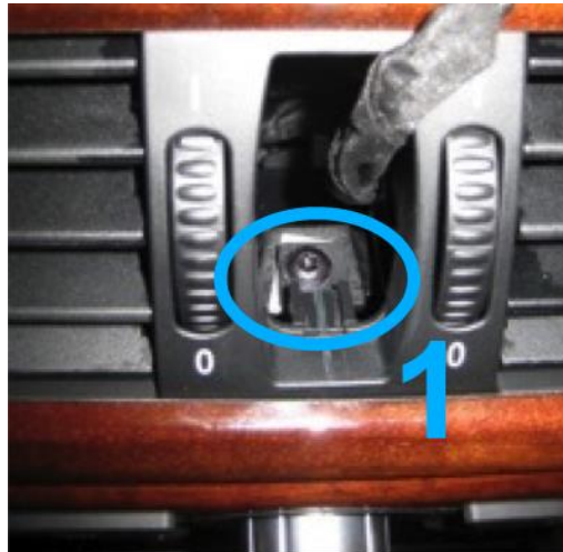
Figure 1 Hazard and Door Lock Switch Screw
