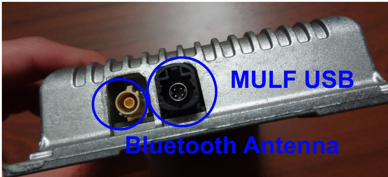
Figure 18 MULF Bluetooth and USB connections
