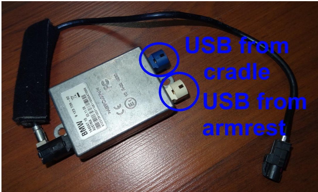
Figure 19 USB Hub originally connected to MULF
