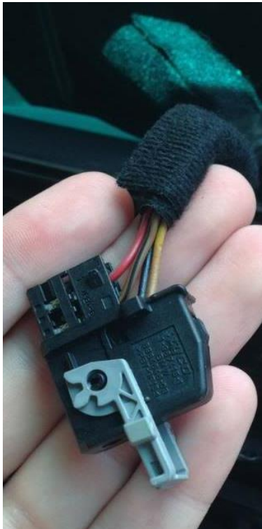
Figure 10 Actual connector slipping out of outer layer
