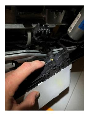
Now the seat controller should be totally free. Go ahead and remove the E92 seat controller using the same process and transfer it over to the M2 seat. All these connectors are plug-and-play and don't need to be modified in any way, so you can just hook them right up on your M2 seat. To keep things simple, plug these connectors back in now before you start disconnecting other stuff on the yellow connector housing. Progress!
