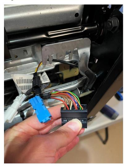
Once you've got your wire migration plan written down (I highly recommend this), start removing the wires from the black E92 connector, and then put the M2 wires into the right spots. It should end up looking like this:
