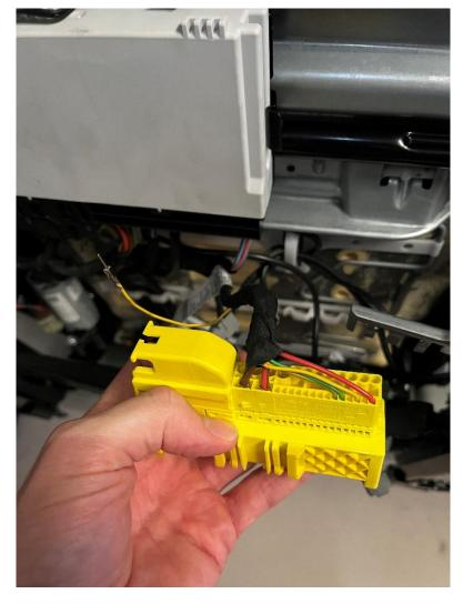
Note that on the passenger seat there is also another single yellow wire on Pin3 that ends with a small grey connector. This is just a loop right back to the harness coming from the floor; function unknown and we won't be migrating this. You can pull the single wire completely out of the wire bundle and discard it. Be sure you're removing the yellow wire in pin3 though. There's the other yellow wire for the side airbags in pin39 (see above) that we're keeping.
