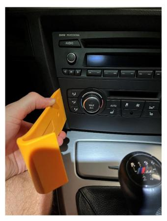
Simply disconnect the cable from the back of the controller. Then work on migrating the faceplate to your new controller. There are 4 clips, 2 on the top and 2 on the bottom (see screenshot below). These are very easy to break, so gently use a trim removal tool to pop the clips.
