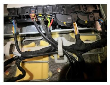
Next, disassemble the yellow connector housing on each seat. This is the most important time to take lots of pictures throughout the process. Within the yellow connectors there are multiple smaller connectors. You will need to cut the zip-tie and then you can gently spread the small yellow clips on the end of the connector, while pushing the grey connector to the side. It will pop out with very little force. We will be re-pinning most of these wires shortly, but don't de-pin any wires yet.
