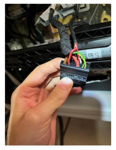
Sidenote: Pins 10-12 on the E92 black connector are used for seat occupancy, and I tried connecting the three M2 occupancy sensor wires (from the small black connector) to these pins. You can see the wires from my attemp on the back row in the pic above, but the car still didn't detect the sensor. Most folks seem to just leave the M2 small black occupancy sensor tied back and unused. If you're curious, the wire pattern I tried (that didn't work) was:
