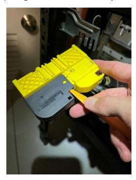
Once the yellow connectors are split apart on both cars, go ahead and remove the seat belt buckle/tensioner from the side of the E92 seat. This is another T50 bolt. Transfer the E92 seat belt receptacle to the M2 seat, and torque the bolt to 42NM (this is important from a safety standpoint). The wiring attached to the seat belt is for the pre-tensioner. Thankfully you don't have to make any changes to this wiring for it to fit right into the E92 yellow connector housing.
