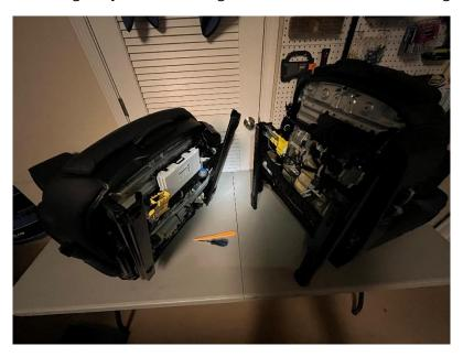
Starting with the M2 seat, remove the seat controller (white box) from its clips under the seat cushion. The side clip is the best place to start. On the back side of the controller, you will find 6 connectors. Go ahead and remove these by flipping down the collars on the big ones and pinching the smaller connectors.
