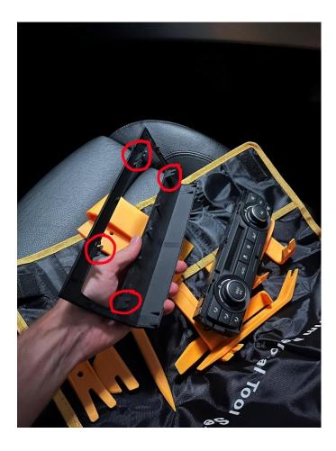
Once you have the faceplate separated, attach it to your new controller, connect the cable to the back, and push it back into your dash.
