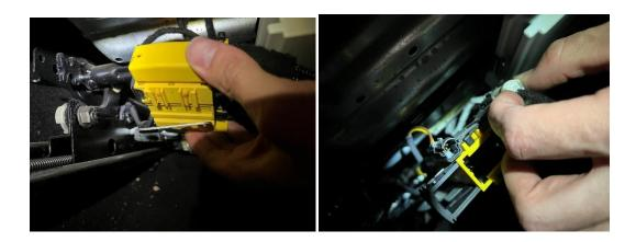
Once the connectors are free, you can remove the seat. I recommend putting towels on the door sill and B pillar, so you don't scratch anything. I'd guess the seat weighs about 50lbs, so you might want a friend to help. This is a good time to vacuum out your floorboard.
