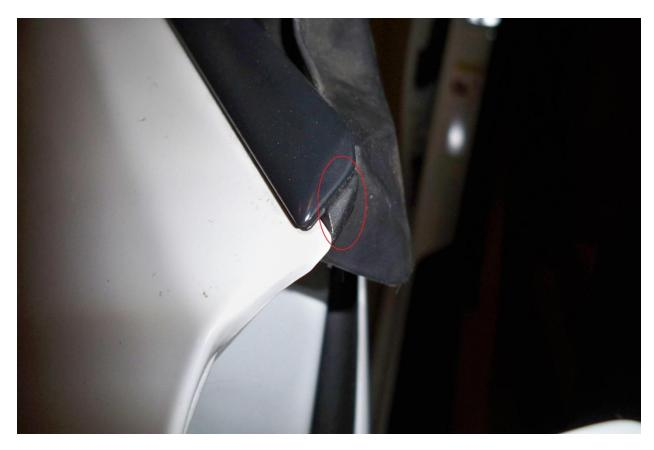
You can now remove the door sill seals with the same method described before. However, there are clips on the front portion of the seals. Just pull the clip forward and slip it over the edge.
