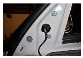
Disconnect the side view mirror wire by squeezing the 2 tabs on the top and bottom of the plug.
