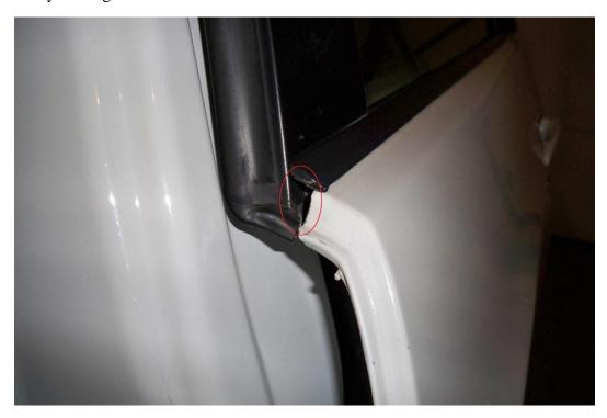
You want to insert the flat-head screw driver into the indicated spot and gently pry the seal up. NOTE: Read on first before prying the whole seal out!
