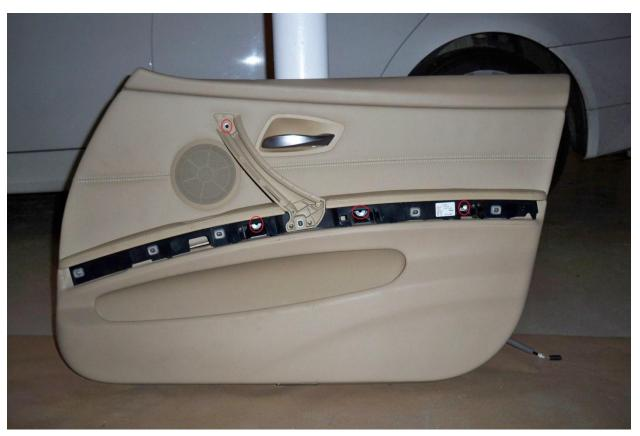
After you have removed the accent trim and hand grip cover from the passenger door, there are 4 T-20 torx bit screws, indicated in red above, that need to be removed. The driver's side door only has 3, located in the same positions above. Now that the torx screws have been removed, the door panel can be pried off the sheet metal. Start at the lower, rear section of the door. You can use the flat-head screw driver to pry it out; just make sure to protect the paint with some tape or a
