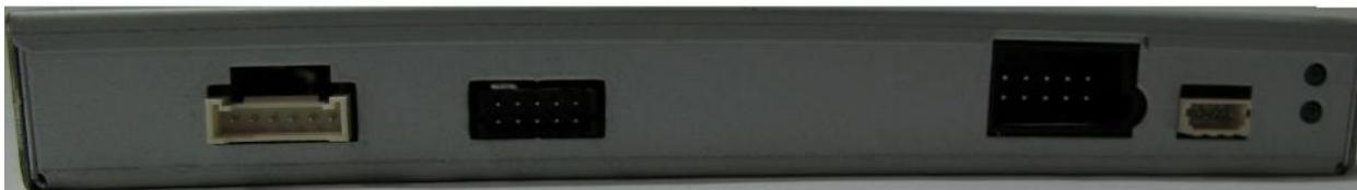
↑ CAN    ↑ LCD-OUT    ↑ LCD-IN    ↑ MODE
