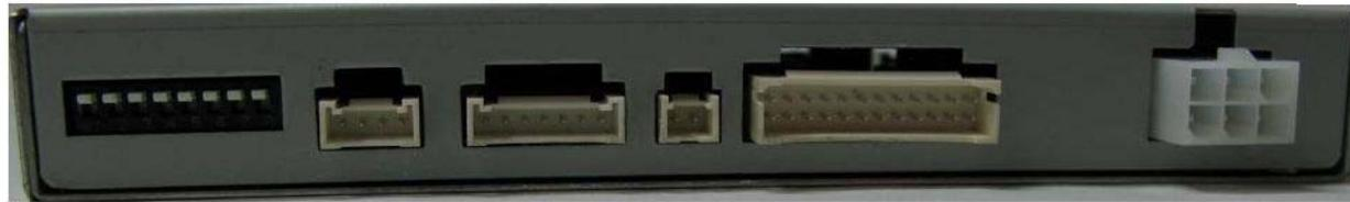
↑ LED    ↑ DIP S/W    ↑ REMOTE    ↑ NAVI IN    ↑ A/V (IN/OUT)    ↑ POWER
