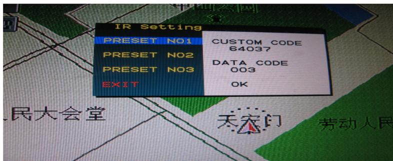
After step No.2, press one button of Navi or DVD remote, then the screen shows the key value and it's saved. Then, you exit IR setting and you can use it right away.
