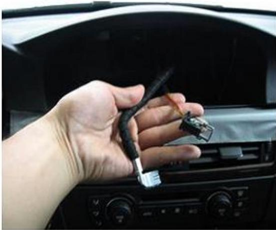
**STEP 5:** Disconnect both cables behind the display unit.
