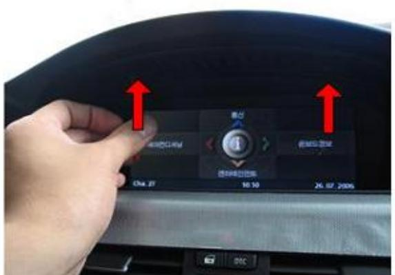
**STEP 2:** Using a small screwdriver unscrew 2 small screws holding upper trim panel.
