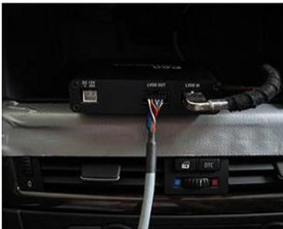
**STEP 7:** Connect Supplied LVDS Cable to LVDS OUT side of the Nav Interface.
