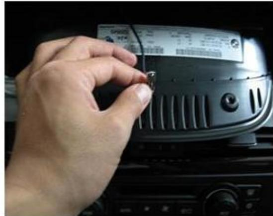
**STEP 12:** Run the wire for the remote eye so that the eye can line up with the remote signal.
