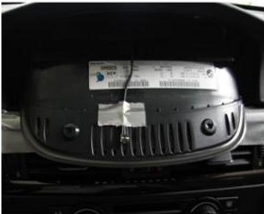
**STEP 13:** Secure the remote eye in a location that it will receive the remote control signal.
