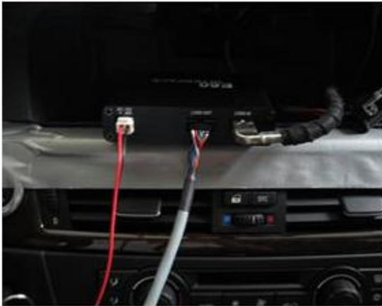
**STEP 11:** Connect the power cable to the Nav Interface Unit.
