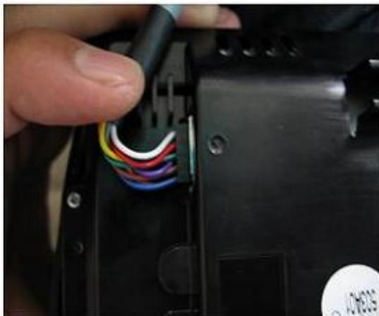
**STEP 9:** Connect LVDS Cable to display part of the in-dash unit.
