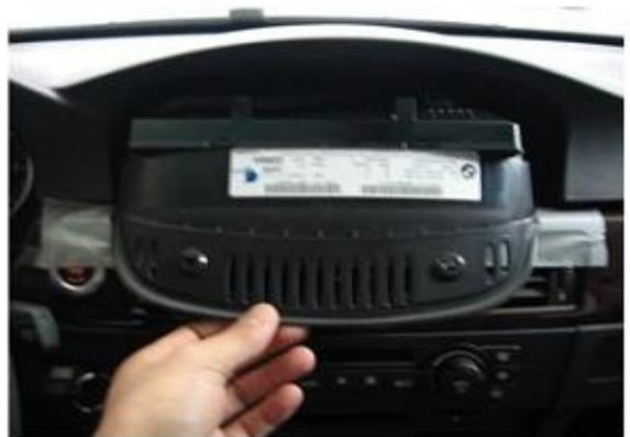
**STEP 4:** Pulling downwards and slightly angling the unit will allow the unit room to come out of dash.
