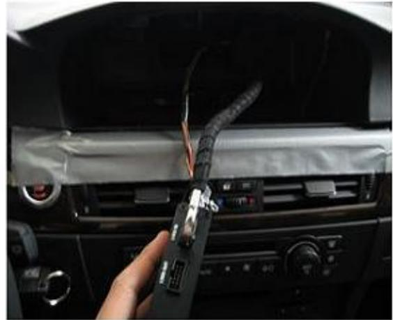
**STEP 6:** Connect LVDS Cable to LVDS IN side of the Nav Interface box.
