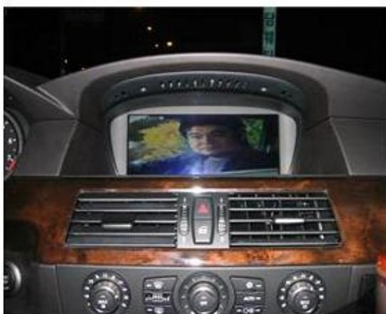
**STEP 15:** Select between the different sources to see if unit shows different inputs.
