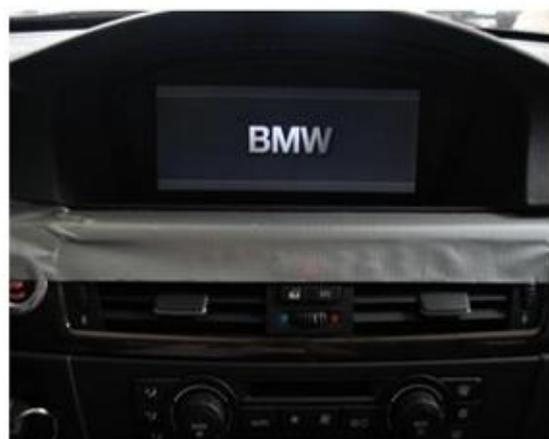
**STEP 14:** Test unit to see if factory display shows on the screen.
