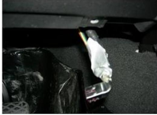
**Note:** When connecting this unit in a BMW 3 Series Car, please be aware that it will be necessary to mount the Nav Interface Unit under the driver's side dashboard using the extension cable supplied.
