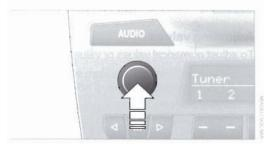
The car radio will select the audio source that was last used: radio, CD player, CD changer\* or external audio device.
