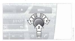
Rotate the right-hand rotary button, arrow 1, to select a menu item, e.g. "TUNER":
