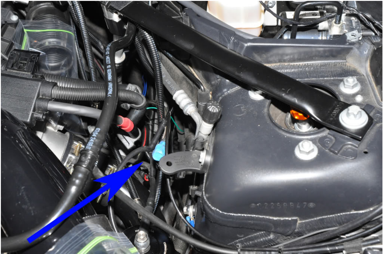
And here is close-up of the NX NO2 fuel line routed into the engine compartment.
