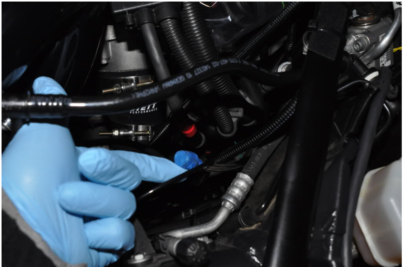
And here is close-up of the NX NO2 fuel line routed into the engine compartment.
