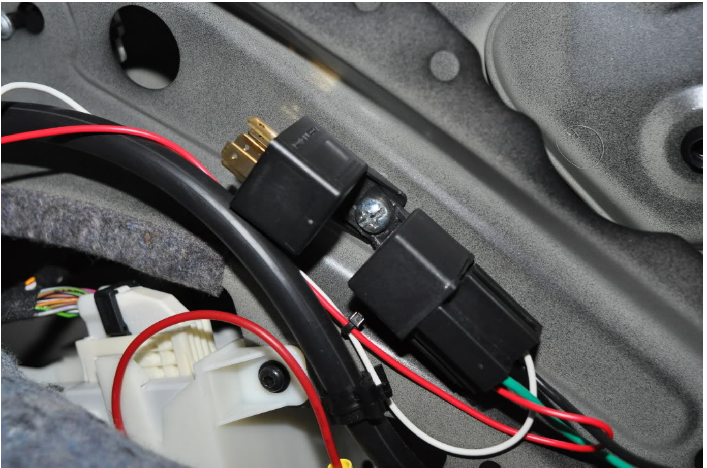
Wire up the relay and label all wires so you know where to hook all the wires up on the switch.
