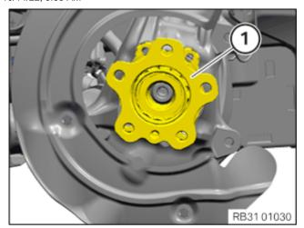
Replacing the front wheel bearing
