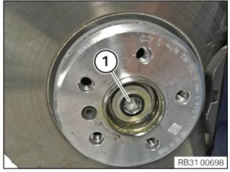
Hand-tighten the collar bolt (1) with the compression spring.
