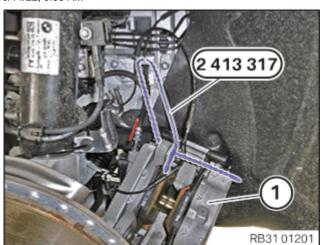
Replacing the front wheel bearing
