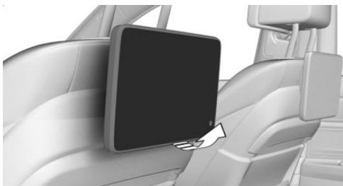
Pull on the bottom edge or press the lower edge in order to adjust the tilt.
