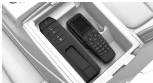
The handset and the snap-in adapter are located in the rear center armrest.
