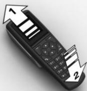
Insert the handset into the holder, arrow 1, and press down, arrow 2, until it engages.
