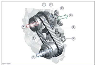
Example transfer box Active Torque Control 13-1
